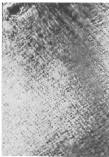
FIGURE 4 Stripe-like textures on an anisotropic phase in ethylene dichloride solution prepared at 37% and 50°C (left) and on a solid film (right) of poly( \gamma -benzyl-L-glutamate) of D. P. 4. — indicates a length of 100 \mu .
